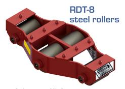
Spikes are 1/2" tall • Bearings are 1/4" x 3-9/16" (15 per roller) • Axles are 1" diameter
